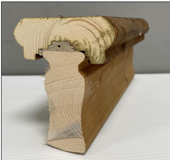
Photo No. 2 Milled Top rail and Handrail
