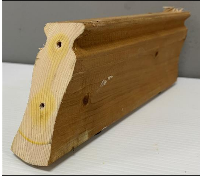
Photo No. 1 Milled Bottom rail
